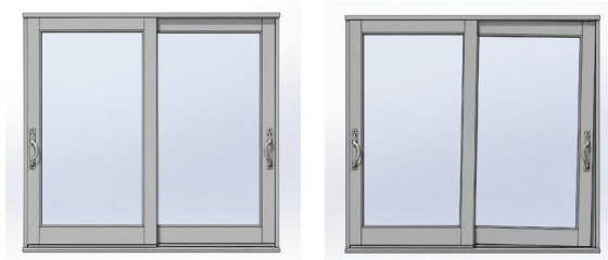
CORRECT PANELS STILES AND FRAME JAMBS ARE PARALLEL
